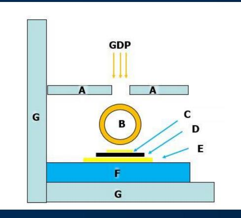
outer diameter (OD) opening with a step height of GDP Capsule R Gel Pak Removable silicon wafer Gel pak
