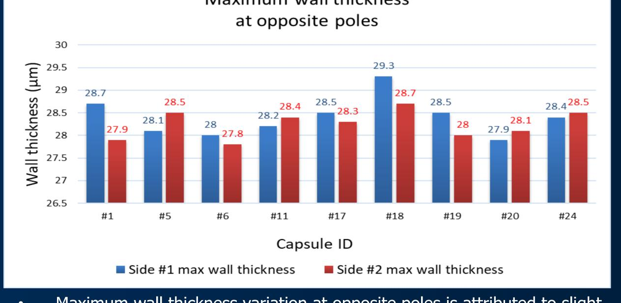
Maximum wall thickness variation at opposite poles is attributed to slight fluctuations in the coating rate during each coating.
